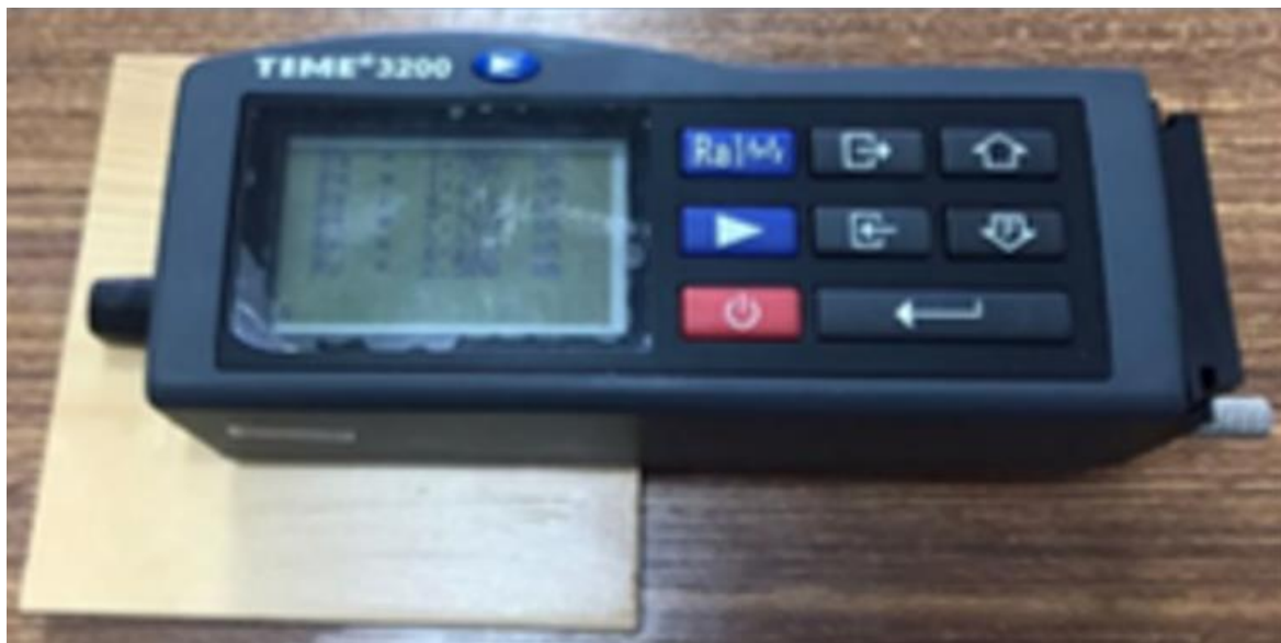
Figure 2. Surface roughness measuring device
