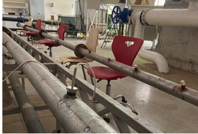
Figure 2: Izmir Katip Celebi University Civil Engineering Department Flow Loop, rough pipe
