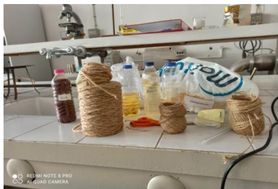
Figure 2. All raw materials to be used in reactive dyeing of cellulosic based natural yarns
