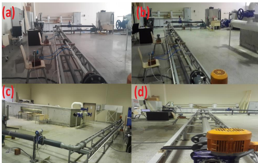
Figure 1. Izmir Katip Celebi University Hydraulics Laboratory (IKCU-CE) Flow Loop including galvanized pipes (a. 40 mm, b. 50 mm, c. 80 mm, d. 90 mm)
